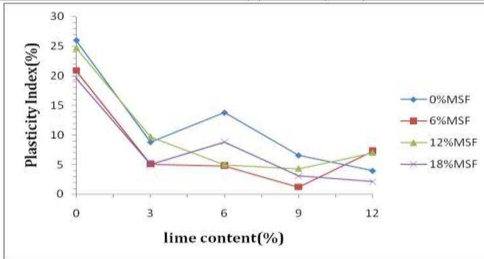
**Figure-5 Effects of L-MSF on the plasticity limits**
