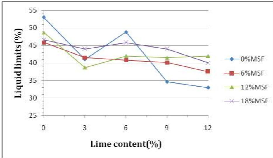
**Figure- 3 Effects of L-MSF on the liquid limits values**
