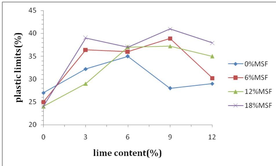
**Figure-4 Effects of L-MSF on the plastic limits**
